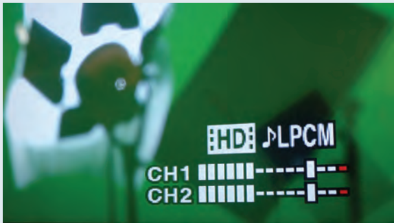
Figure 9.11 Use the sound levels display function on the camera so that you know you are definitely recording and that your sound levels are appropriate.
