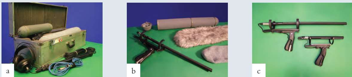
Figure 9.10 (a) Road case and microphones suitable for FTVNM students to borrow. Good sound can make all the difference to your productions. (b) Sennheiser MK 816 microphone and a selection of wind baffles – from top: a ‘zeppelin’, a ‘dead cat’ and a ‘windsock’. (c) Sennheiser MKH 816 and 416 microphones. These have a super cardioid recording pattern.
